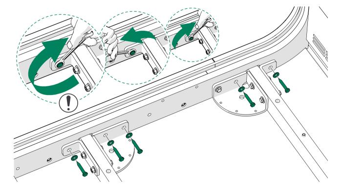
**5.** Fasten the bolts (16 pcs) in the support board with SW13.
