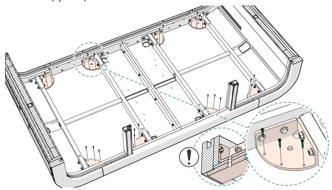
3. Screw in the leveling feet to lower the pod.
