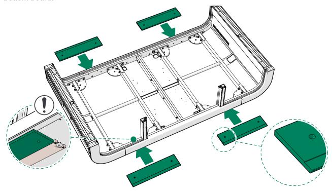
2. Screw in the plywood pieces with 4x30 screws.
