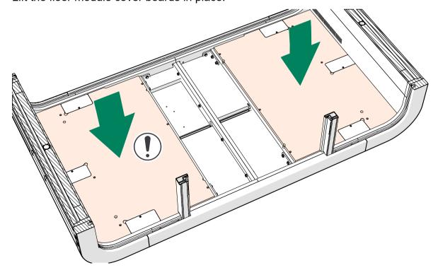
3. Screw the floor module cover boards back into place with 5x50 screws (12 pcs).
