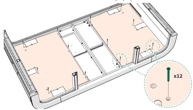
2. Remove the floor module cover boards by lifting them upwards.
