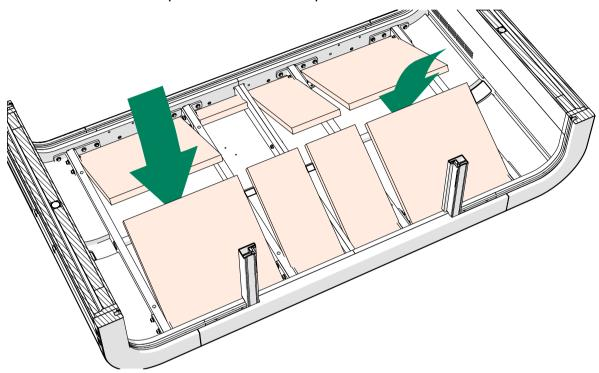
2. Lift the floor module cover boards in place.
