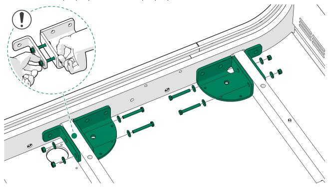
2. Fasten M8x70 bolts (4 pcs) and ST 9.5 washers in the holes where the metal springs are located inside the frame.
