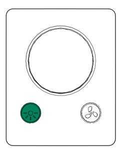
2. Rotate the control disc clockwise to brighten and counter-clockwise to dim the light.
