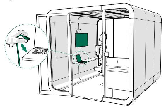
4. If equipped with the optional LAN cable, connect the LAN cable to your laptop.
