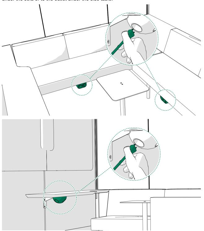
**3.** In 2Q Huddle, connect the power plug to the power outlet on the table or to the outlet under the table.
