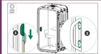
Do not overtighten the handle screws.
