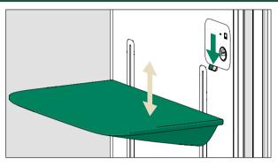
• If the table does not move smoothly or to the maximum height, reset the table.
