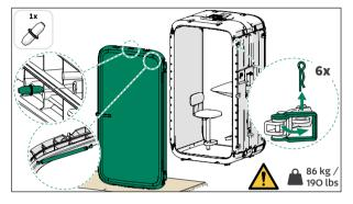
Make sure that the door frame is the right way around. The strut should be in the upper corner.
