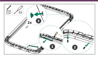
(1) Change the door handedness if necessary before installing the door.
