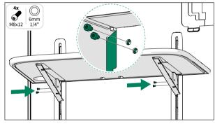
• Install the screws from the left side of the table brackets.
