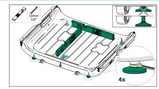
$\begin{tabular}{l} \P \end{tabular}$  If the floor is not leveled, the sound insulation of the pod will be improper. Level the floor and after leveling, stand on it to make sure that it is stable.
