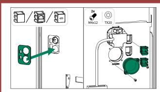
If LAN cord or USB-C module (options) are included, install the keystone connectors and connect the LAN or USB cords.
