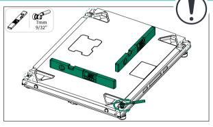
If the floor is not leveled, the sound insulation of the pod will be improper. Level the floor and after leveling, stand on it to make sure that it is stable.
