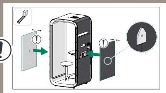
• The thinner acoustic panel is for the table wall and thicker for the back wall.
