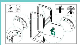
Make sure that the fan cables or the roof module seal do not get pinned between the roof module and pod frame.
