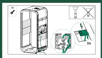
1. HDMI cable from the roof to the touchscreen 2. 24V cable from the roof to the power unit
