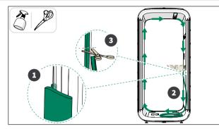
(i) Use glass washing liquid as a lubricant to help install the gasket.
