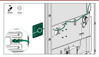
Test the electrics. Connect the power cord and verify that the touchscreen and both lights turn on. Disconnect the power cord.
