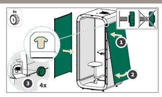
• The smooth side of the fastener must point outward.
