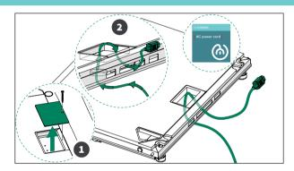
• If the power cord is routed through the roof, continue to the next phase. The power cord is installed later after connecting the electrics.
