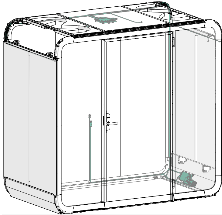
Figure 4: Overview of the pod electrics
